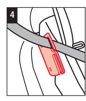
Secure the shoulder belt through one of the notches in the shoulder belt positioning guide. The belt should cross the base of the child's neck and across the chest (not the face or neck). Pull up on the shoulder belt to tighten.
